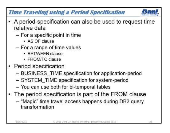
Queries against temporal tables can also contain a clause called a periodspecification. This period-specification can be for a specific point in time, or for a range of time values. However, it is important to know how the queries will behave both with and without the time specification.
