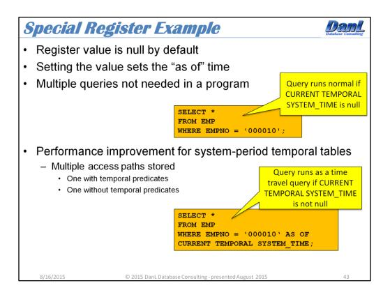
Using these special registers allows for only one query to be coded against a temporal table. Whether or not that query is a normal query or time travel query is then dependent upon the special register setting. Setting the special register to the null value will cause the query to execute as if there was no period-specification, and any valid non-null value will cause the query to execute as an "as of" time travel query.
