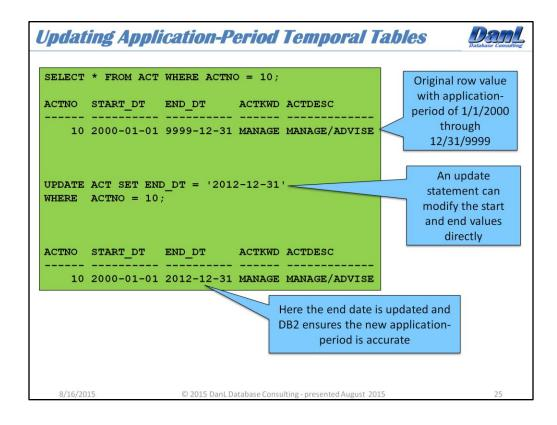
You can execute normal insert and update statements, but if the unique or primary key of the table includes the business time then your insert can add a row for an already existing non-time based key value and a delete could remove multiple rows representing different time ranges for a value. Our ACT table has a non-time key column of ACTNO and then the time duration as part of its unique key. Inserts, updates, and deletes will have to consider the time duration.
