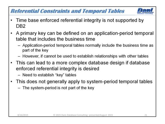
Time based referential integrity is currently not supported by DB2. So, while you can define a primary key on an application-period temporal table, you cannot establish relationships with other tables. Since the whole point of application-period temporal tables is to add a time component to what was otherwise a primary key this adds some considerations and complexity to a database design that utilizes application-period temporal tables.
