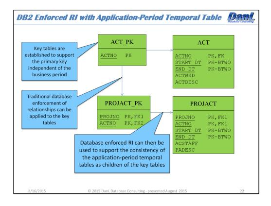
One solution to the challenge of database enforced referential integrity for an application-period temporal table is to establish separate key tables that support the database enforced referential integrity, while their application-period temporal children support the storage of the detailed elements.
