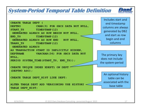
When you define a system-period temporal table DB2 is completely in control of the start and end timestamps. The timestamps reflect the period of time in which the data is current, and are not part of the primary key. This history table is optional, but when defined and related to the base table DB2 will automatically propagate "before" images of any data that changes to the history table and include the proper start and end timestamps.
